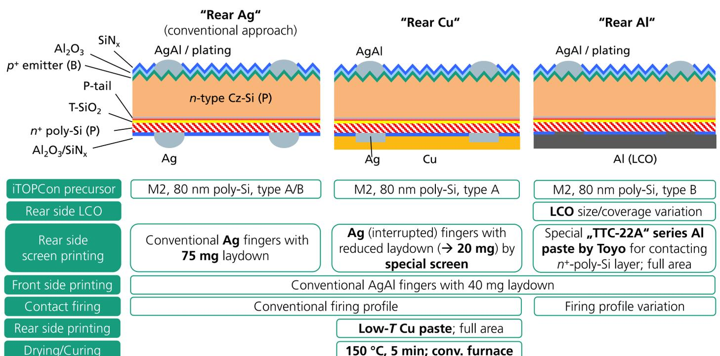
iTOPCon cross-sections and corresponding rough process flows
