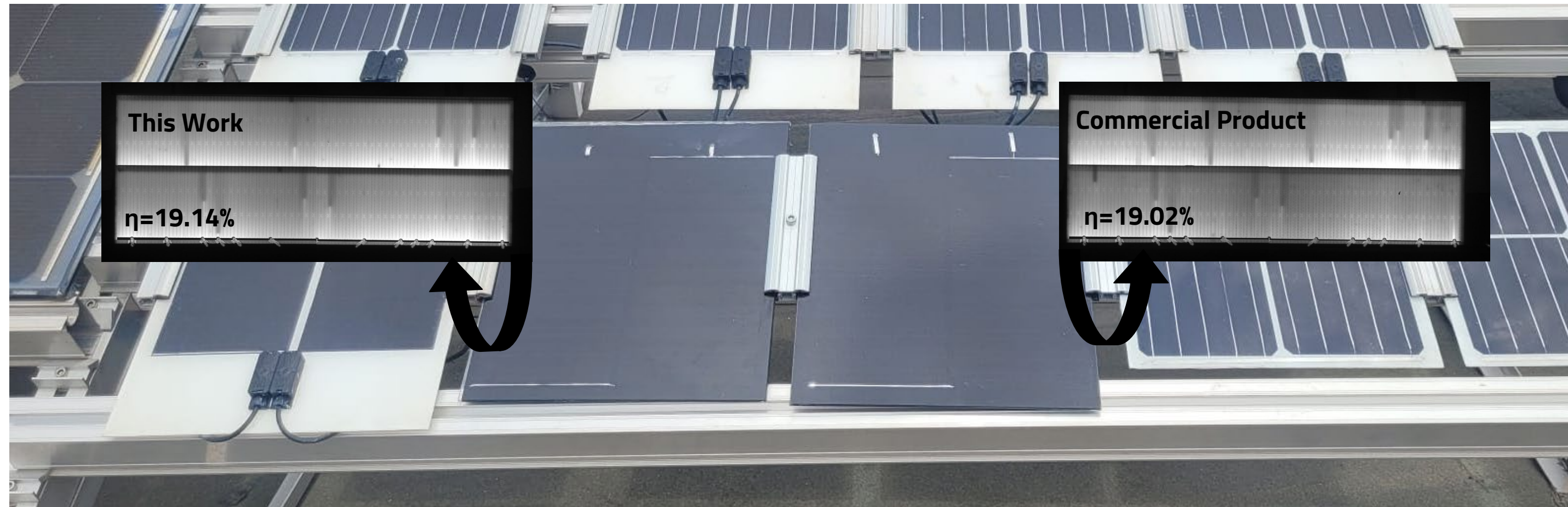
Electroluminescence and Field Testing of Water-Based and Commercial ECAs.
