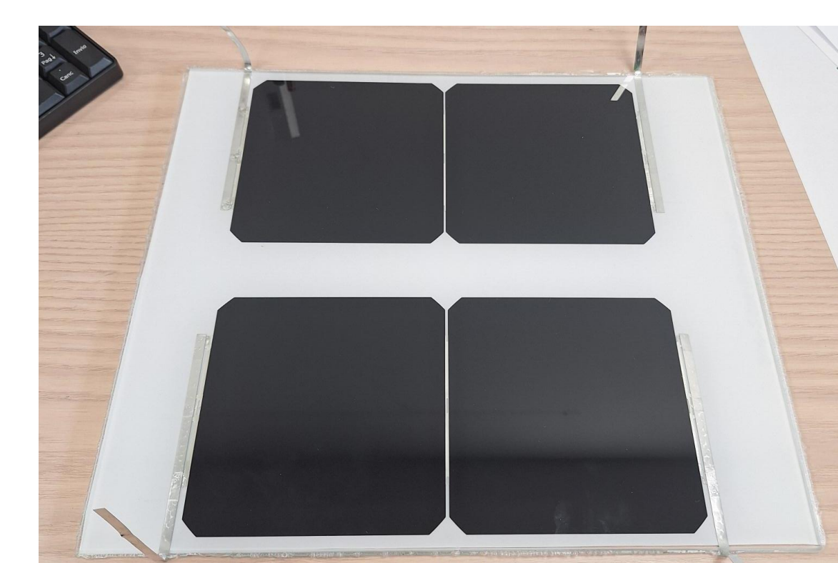
Figure 5: Mini-modules of 2 cells interconnected with ECA-UV, after lamination.
