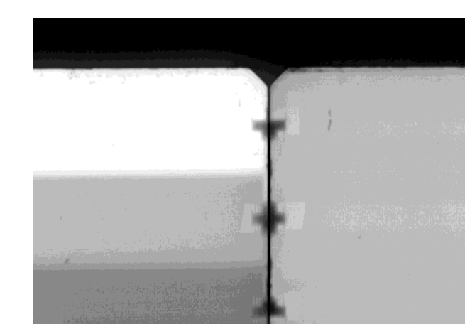
Figure 6: EL with intensity changes per connected area, associated to different connection resistances.
