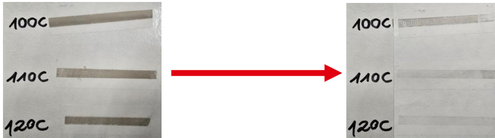
Tack-free samples after 20s at 120 °C
