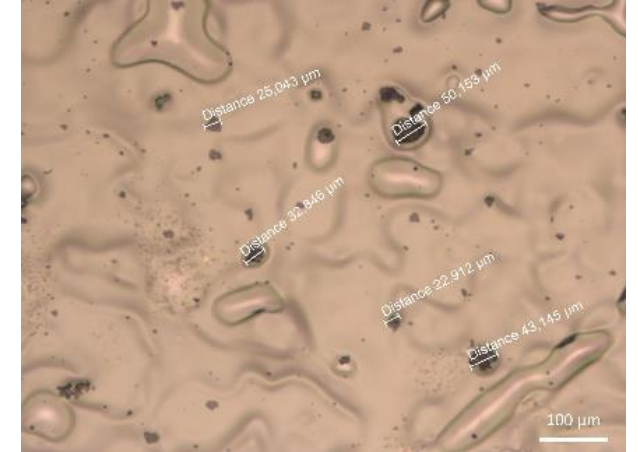
ECT3: 10 μm-thick; anisotropic tape with acrylic adhesive filled with Ni particles.
