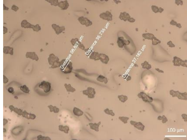
ECT2: 50 μm-thick; anisotropic tape with acrylic adhesive filled with Ag particles.
