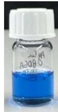
AgCu + solvent+ HD1 (Post particles filtration)
